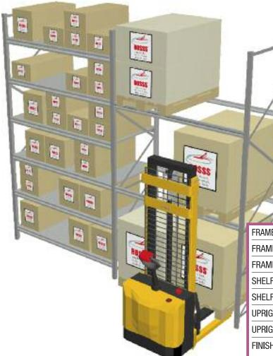
FRAME MAX LOAD CAPACITY 8.400 Kg FRAME MAX HEIGHT 9.00 mt FRAME MIN HEIGHT 1,80 mt SHELF LENGHTS from 1000 mm to 2700 mm SHELF DEPTH from 400 mm to 1400 mm UPRIGHT DIMENSIONS 60 mm **UPRIGHT STEEL THICKNESS** 1,2 - 1,5 mm **FINISHING** hot galvanized sendzimir
